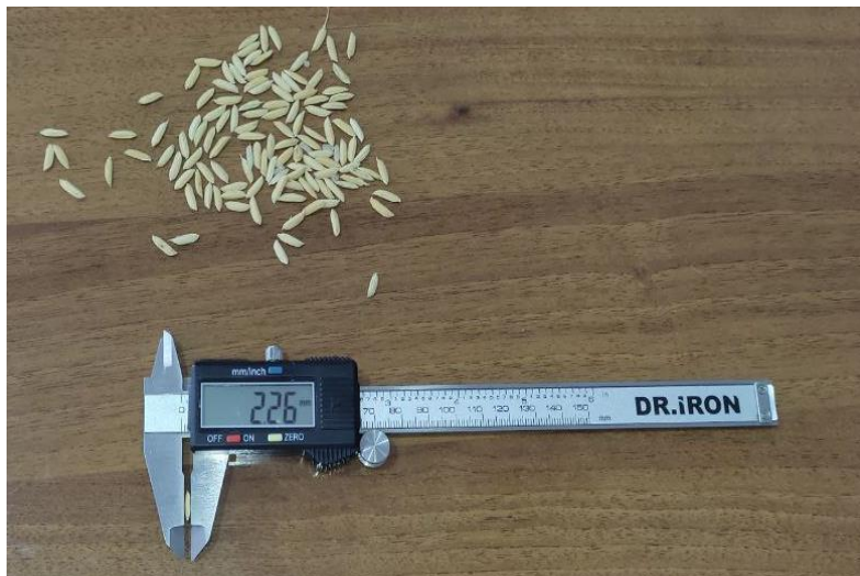
2-rasm. Sholi donasini geometrik o'lchamlarini o'lchash jarayoni
