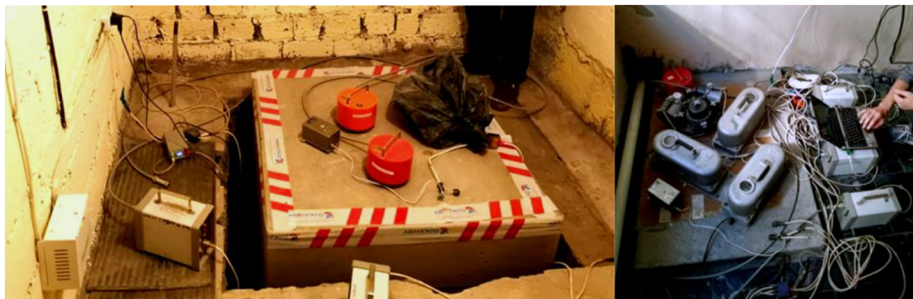
Figure 3. Seismic stations “Karmadon” (on the left) and “Vladikavkaz” (on the right), where sensors IGES-006 and SPV-3K were installed.
