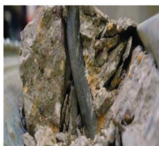
Fig. 5 (b) shear failure of stud
