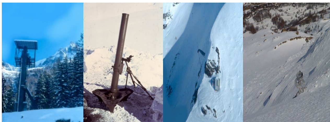
Figure 13. Artificial avalanche release methods with avalanche cannon, CATEX, GAZ-EX, and AVALHEX blasting methods [ANENA, 1994].
