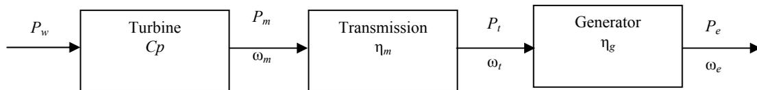
Fig. 5. Wind electric system
